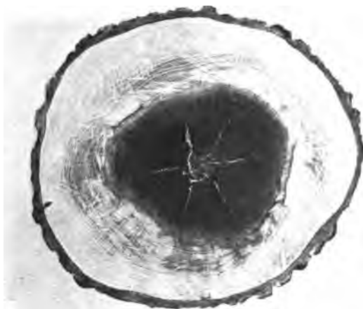
Cross-section of oak showing work of Polyporus sulphureus (Bureau of Plant Pathology, Bulletin 49)
